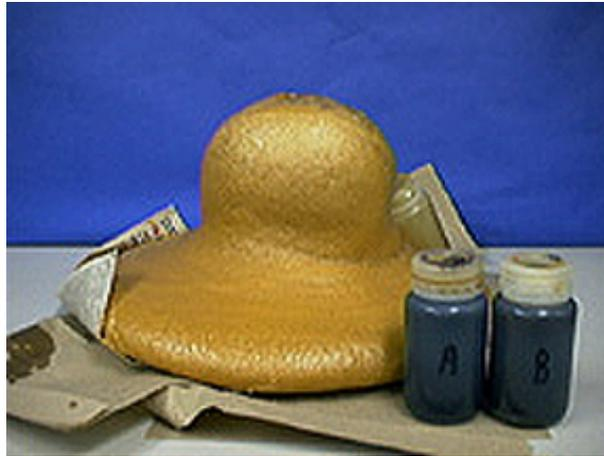
Fig. 1 Final shape of a polyurethane foam after mixing of products A (isocyanate) and B (polyol).
