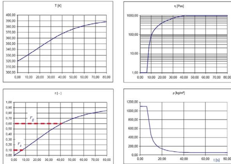
Fig. 2 Evolution of temperature, viscosity, reaction rate and density during the expansion process.
