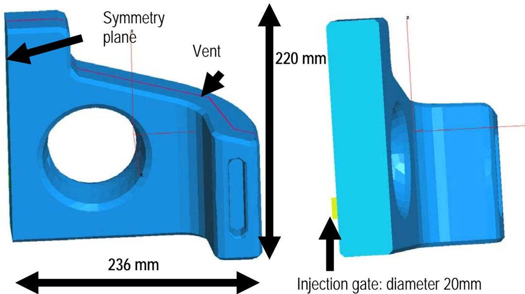
Fig. 5 Half geometry of the demonstration case.
